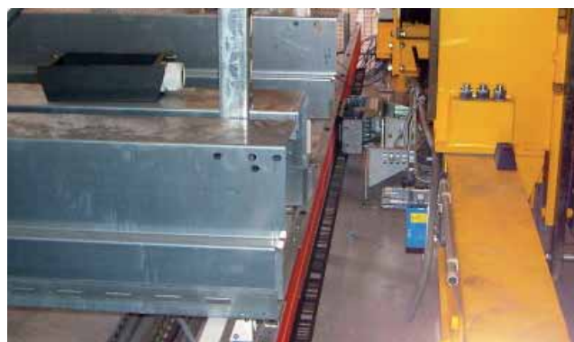
Application of a 10-pole Pro-Ductor system with code rail
